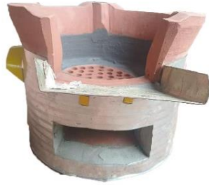
Figure 2: Photo of Lao Energy Saving Improved Cookstove
